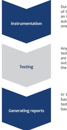
During compilation, Testwell CTC++ automatically instruments a copy of the source code by injecting measurement code. This creates an instrumented version of the program or test executable – fully automatically during the build process or on the basis of a simple, one-time build configuration.
